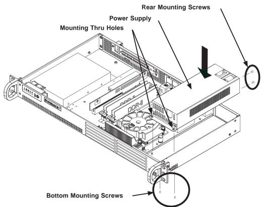
Figure 6-5. Installing the Power Supply
